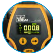
Displays neutral to ground voltage
