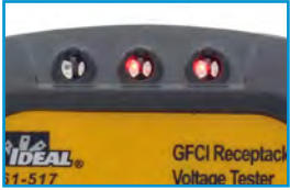
Red Lights Indicate Incorrect Wiring
