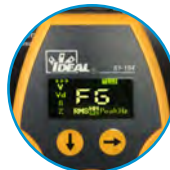
Detects and Displays false or "bootleg" ground
