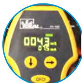
Trips GFCI at 6mA or 30mA
