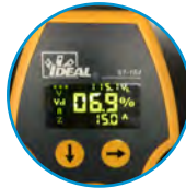
Displays Voltage Drop at 12, 15 & 20 Amps
