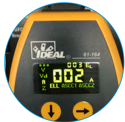
Estimated Load on Line in Amps
